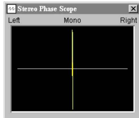
STEREO IMAGE SCOPE — USE THIS MODE WHEN MIXING MUSIC/SOUND. PAN AND DIRECT YOUR AUDIO SIGNAL SOURCES IN THE STEREO SOUND FIELD. ALSO VERIFY MONO COMPATIBILITY. IN THIS VIEW L/R SIGNAL ARE PANNED TO THE CENTER EQUALLY.
