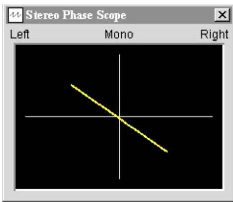
MISSING CHANNEL SENSOR — THE SCOPE PATTERN ABOVE INDICATES LOSS OF RIGHT CHANNEL INPUT SIGNAL. THIS IS ALSO WHAT THE DISPLAY WOULD LOOK LIKE IF YOU PANNED A SIGNAL SOURCE TO THE LEFT.
